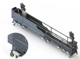
The  $CoxGomyl^{TM}$  Modular Self Powered Platform is the ideal choice for safe and efficient facade access for up to three operators. The platform has been re-designed and constructed from lightweight aluminium in combination with perforated panels. It can be assembled to obtain the platform length required on site thanks to its safety pin system.
