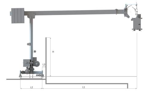
Often referred to as a 'crane type' Building Maintenance Unit (BMU), the CoxGomyl™ F3000 is used when the reach or suspended load is increased beyond the capabilities of the E-type machines. This economical BMU has an impressive higher load capacity of 500 kg for the auxiliary hoist and a reach of up to 14 metres, and is manufactured within 12 weeks or less for any machine in the range.
