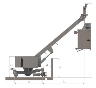
The CoxGomyl™ E3000 Building Maintenance Unit (BMU) is a reliable and great value solution for buildings of lower height and uniform shape. A compact, robust and lightweight machine, the E3000 is almost entirely hidden from sight from ground level when not in use. Due to its compact profile, the E3000 machine is particularly well suited to applications with limited space on the roof and buildings with roof gardens.
